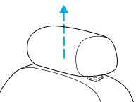
Push control to lower head restraint.
